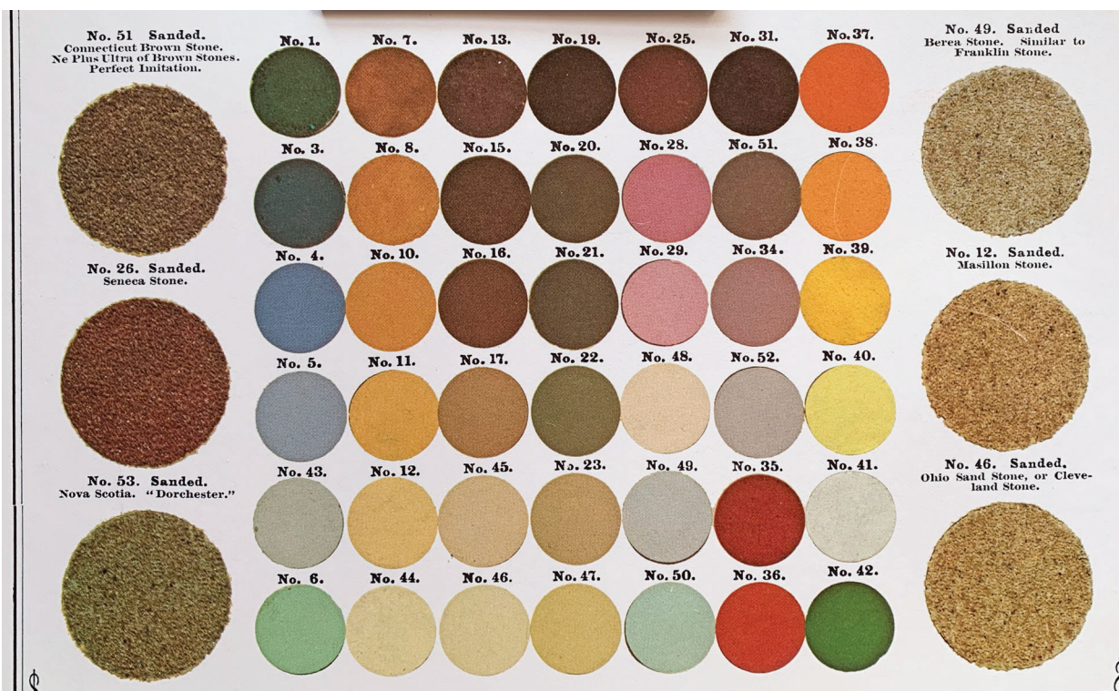
1880s color chart by Harrison Bros. & Co. with sanded paint samples on the right and left sides. The labels above the samples include the type of sandstone being imitated.
